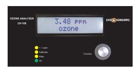
The Eco Sensors model UV-100 ozone analyzer is for general purpose measurement of ozone in air. Its range is .002-100 ppm (v) with 2% accuracy, and it includes a built-in data logger. The UV-100 weighs only 2.1 kg (4.7 lb), it is powered by an AC adapter or 12 V external battery, and is equally versatile for the laboratory
